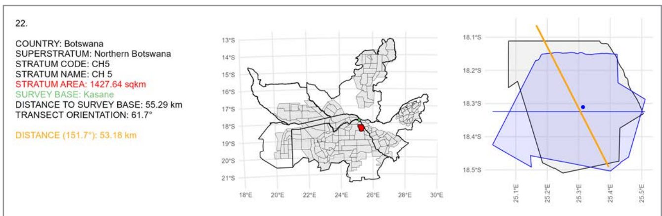
Figure A2.1: Calculation of the length of the baseline for stratum CH5 in northern Botswana.
